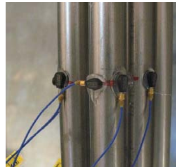
Fig. 83 Sketch of the tubes tested and real position of the accelerometers
