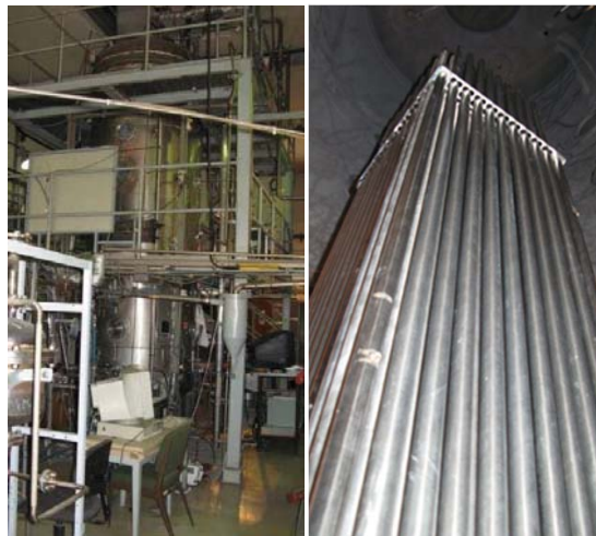
Fig. 6 The LASS facility with the PECA vessel at the bottom. Right: The tube bundle view
