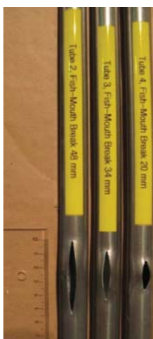
Fig. 24 Fish-mouth breaches: 1D, 0.5D, 0.25D
