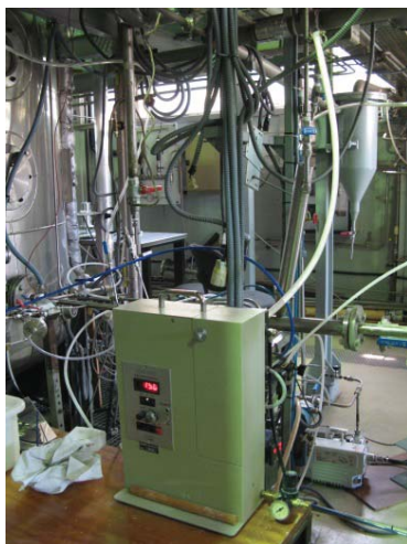
Fig. 56 RGB-1000 aerosol generator used for the AAA tests
