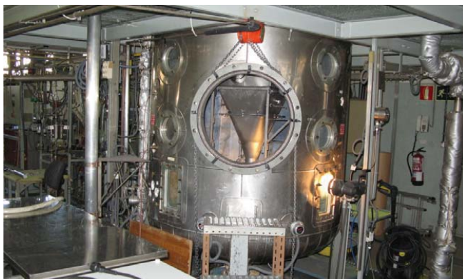
Fig. 54 Outside view of the MSAA within the PECA vessel
