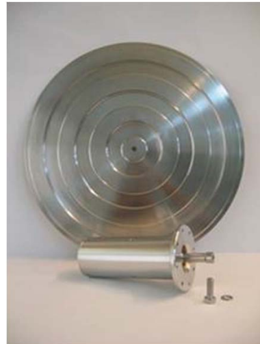
b) View of the circular radiating plate, the ultrasonic vibrator and the bolt mechanical pre-stressing
