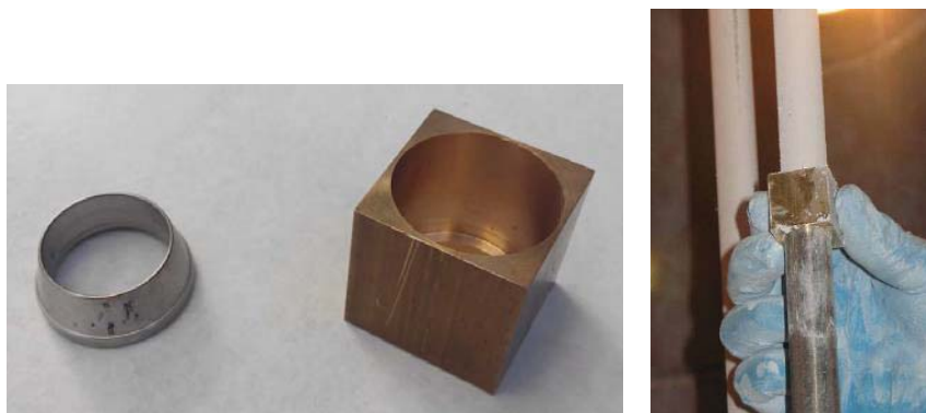
Fig. 22 Left: U-ring; bevelled bi-cone and squared nut Right: Collection of particles along a tube
