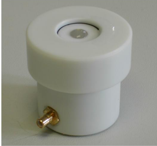
Fig. 7. Sensor-cell for experiments with liquids.
