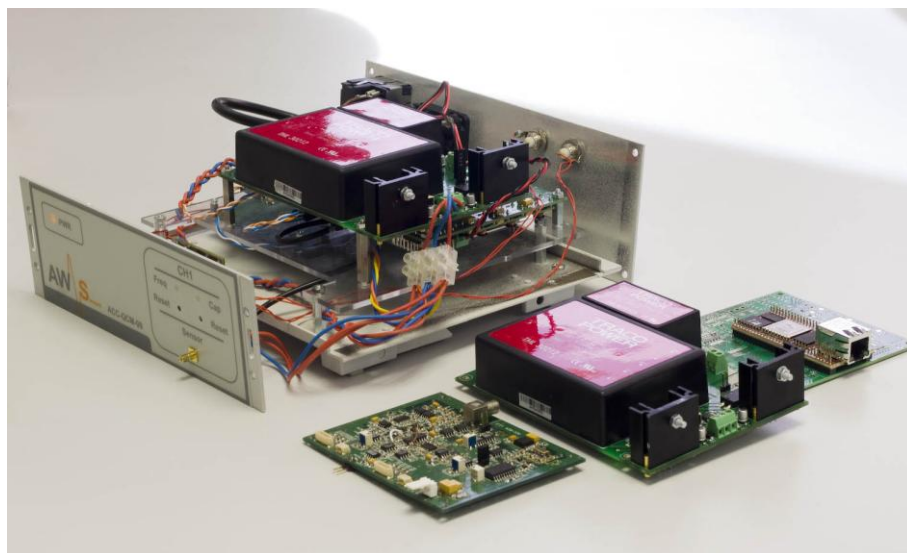
Figure I.39. ACC-QCM-09 Instrument. Subsystems assembled and distributed inside the enclosure.
