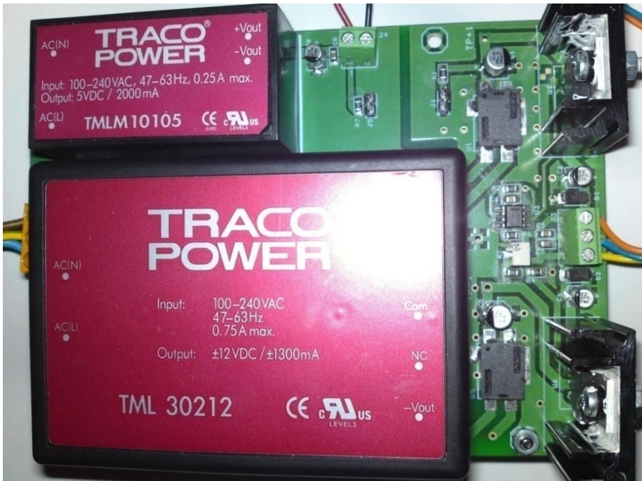
Figure I.38. Assembled Power supply circuit.
