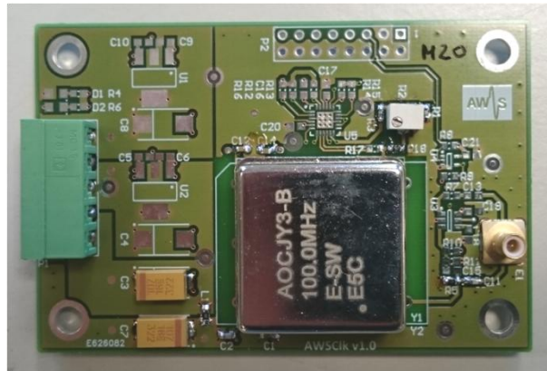
Figure II.5 DDS reference clock board. The circuit was designed to be compatible with two different 100 MHz high performance OCXOs: the AOCJY3-B from Abracon LLC. and the O-3311AT from KVG Quartz Crystal Technology GmbH (Abracon Corporation, 2011; KVG Quartz Crystal Technology GmbH, 2007). Although it is common to find 10 MHz high performance OCXO-based reference clocks, the selected output frequency was 100 MHz. We opted for this frequency to minimize the phase noise multiplication factor introduced by the PLL clock multiplier (Calosso et al., 2012; Rubiola, 2010). We were able to work at the highest sample rate of the DDS (500 MSPS) with a low PLL factor of 5, minimizing the signal generator system's phase noise introduced by the reference clock.
