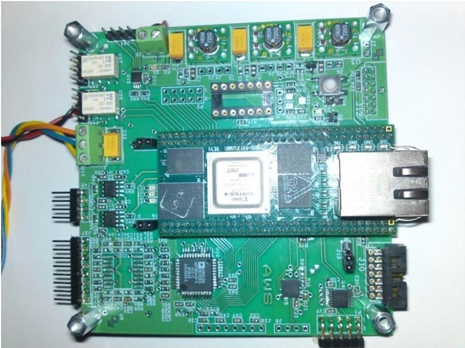
Figure I.35. Assembled communications and data acquisition circuit. Top view.
