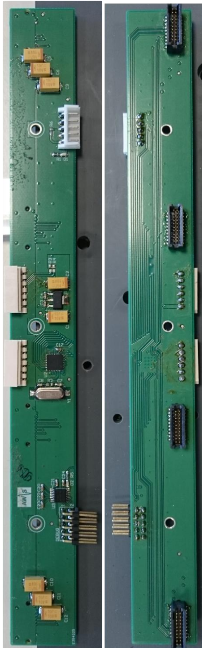
Figure II.16. Assembled bus adapter circuit. Top and bottom views.
