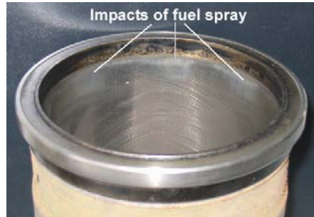
Figure 2.12. Cylinder liner wear due to spray impingement during early pilot injection. Source: Dronniou et al. [47].
