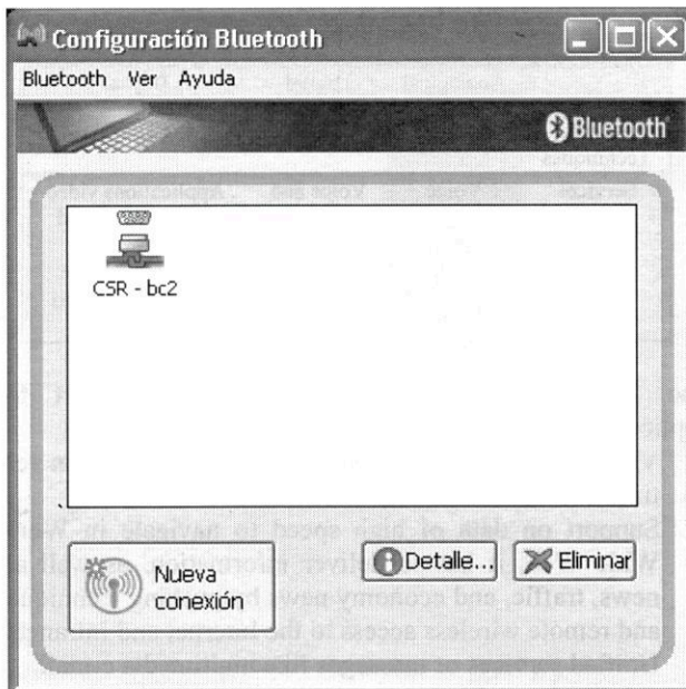
Figure 15. Aspect of the configuration dongle window when BC02 module is connected to the dongle.
