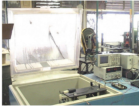
FIGURE 16 Photograph of the visibilimeter during calibration procedure. (color figure available online.)
