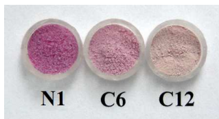
Figure 2 Changes in colour observed in N1 nanoparticles in the presence of certain carboxylates. From left to right: no carboxylate, hexanoate and dodecanoate
