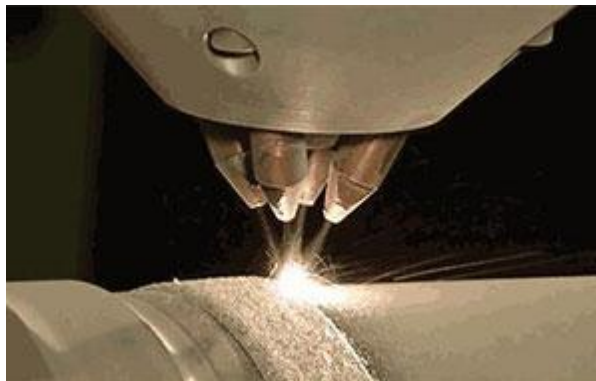
Figura 3-33 – Processo LENS da Optomec ( Laser Engineered Net Shaping ) 139
