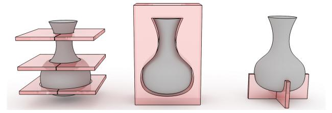
Fig. 2. Different types of tailored housings. (left) Rigid foam template packing. (center) Cavity packing. (right) Cradle mounts.
