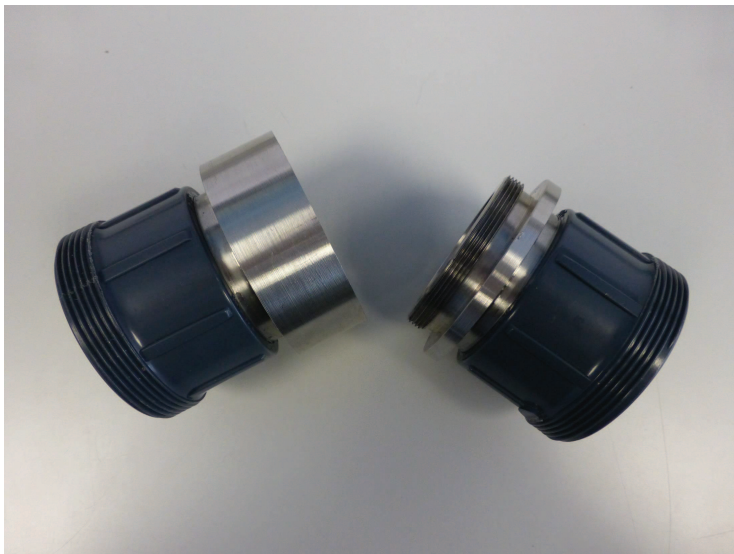
Figure 3.6: Sample holder for the study of the sintered plates.
