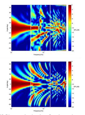
**Fig. 19** Diagrams showing the reflected acoustic pressure field (Sound Pressure Level - SPL) of the  $\theta_{MOP}$  3 individual as a function of the angle and the frequency calculated using both FDTD (above) and Fraunhofer theory (below). Vertical white lines delimit the frequency range in which diffusers have been optimized in this work.
