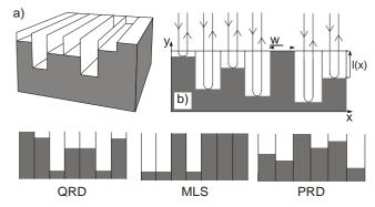
**Fig. 1** (a) A scheme of 1-D Schroeder diffuser; (b) Explanation of the acoustic response of these diffusers; (c) Sectional views of QR, MLS and PR diffusers. *l*(*x*) represents the depth profile of the diffuser. *W*is the width of each well.
