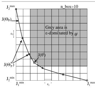
**Fig. 5** The concept of s-dominance in a bi-objective problem.  $J(\Theta^*)$  is the smart characterization of the Pareto front  $J(\Theta_P)$ .  $J^{min}$ ,  $J^{max}$ ,  $J^{max}$ , Pareto front limits;  $s_1 = (J^{max} - \frac{1}{J^{min}})/n$ -box,  $s_2 = (J_2 - J_2)/n$  boxbox widths; and n box, number of boxes for each dimension.
