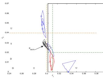
Fig. 8 Pareto Front for MOP1 with the preferences ranges and the selected diffuser  $\theta_{MOP1}$ . Analysis of performance degradation.
