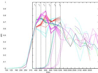
**Fig. 10** Frequency Response for MOP2. Solid lines: Optimization range. Dashed lines: Out of the optimization range. Notice that frequencies over 1332Hz are over the limit of validity of the Fraunhofer theory.
