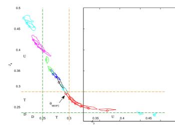
Fig. 11 Pareto Front for MOP2 with the preferences ranges and the selected diffuser  $\theta_{MOP2}$ . Analysis of performance degradation.
