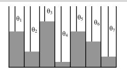
**Fig. 3** Profiled diffuser with seven wells. Well width w = 0.9/7 = 0.128m. Maximum depth of each well 0.32m.
