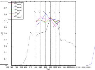
**Fig. 18** Frequency response comparative for  $\boldsymbol{\theta}_{MOP1}$ ,  $\boldsymbol{\theta}_{MOP2}$ ,  $\boldsymbol{\theta}_{MOP3}$ ,  $\boldsymbol{\theta}_{QR}$  and  $\boldsymbol{\theta}^*_{MOP2}$ . Solid lines: Optimization range. Dashed lines: Out of the optimization range. Notice that frequencies over 1332Hz are over the limit of validity of the Fraunhofer theory.
