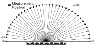
**Fig. 2** Schematic measurement set up to obtain the diffusion coefficient of a sample composed by an array of four diffuser. Each diffuser has a width of 0.9m. Then  $X_L$  in Eq. (1) is 1.8m. The wells width is w = 0.9/7 = 0.128m.
