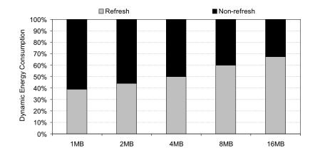
Figure 1: Dynamic energy split into expenses due to refresh and non-refresh operations in eDRAM technology, varying the aggregate L2 capacity.
