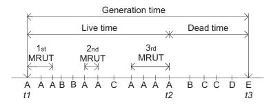
Figure 2: Generation time of the cache block A.
