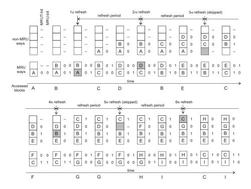
Figure 8: Example of periodic refresh operations performed by *Cond* in the devised energy-aware cache.
