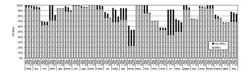
Figure 11: Hit ratio (%) of the *enaw* cache, divided into hits in MRU and non-MRU banks for the refresh policies considered.
