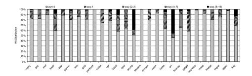
Figure 4: Percentage of cache hits across the ways of a 128B-line 2MB-16way L2 cache using LRU replacement.
