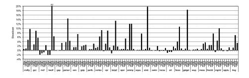
Figure 12: Slowdown (%) of the phased cache and the *enaw* cache for the proposed refresh policies with respect to the conventional cache.
