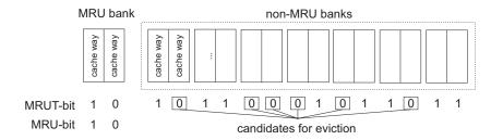
Figure 6: Diagram of the data array of the *enaw* cache with the control bits of the MRUT algorithm.
