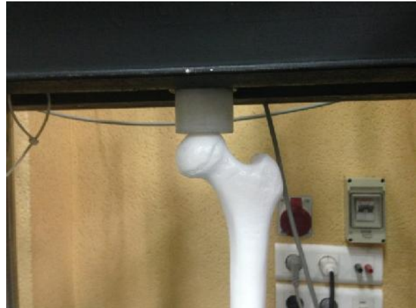
Figure 2. Upper fixture support.
