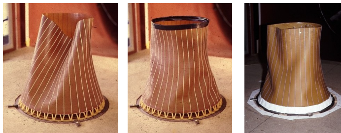
Fig. 10: Models Without and With an Upper Edge Ring ; Model With Internal Suction [7].
