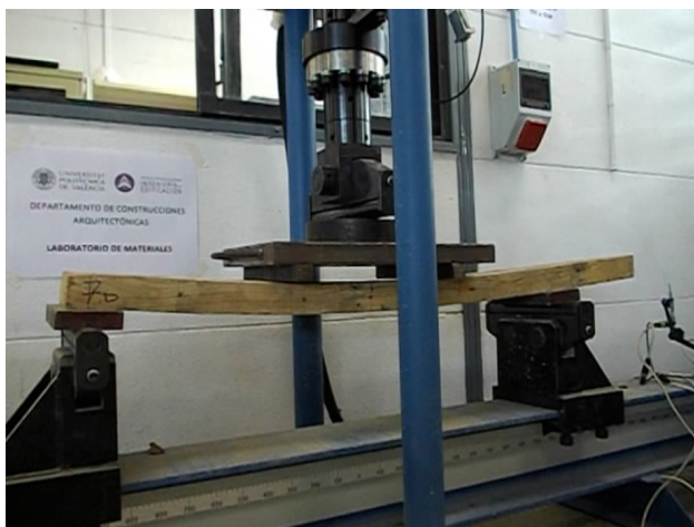
Fig. 12 _Dismantling of sensors and application of the load till break
