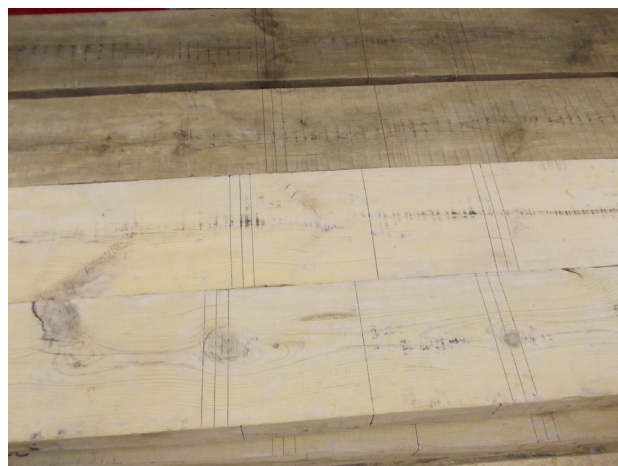
Fig. 7 _Drawings of reference lines for the application of loads and of sensors
