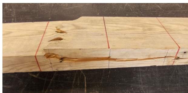
Fig. 14 _Structural failure of element n.8, view from above
