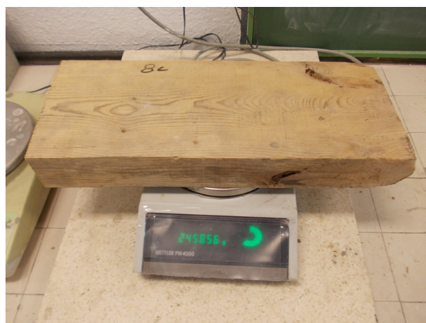
Fig. 16 _Measurement of the mass of a specimen for the calculation of the density
