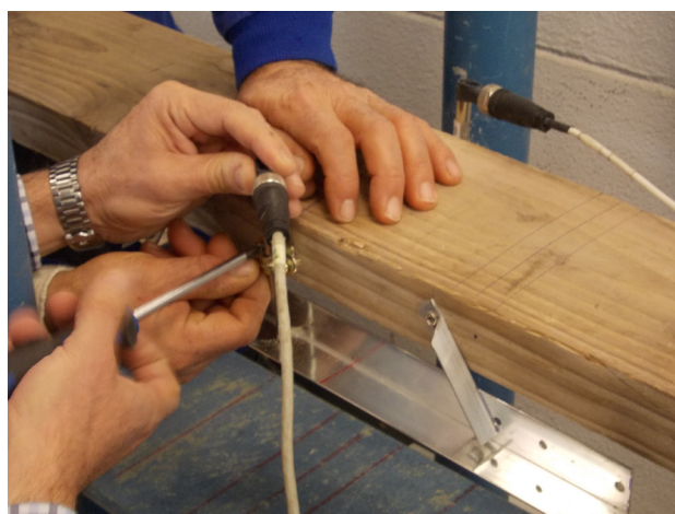
Fig. 8 _Monting of metal supports and positioning of sensors for the measurement of local modulus of elasticity
