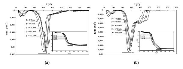
Figure 1. TG (inset) and DTG curves for rice straw under inert (0 %  $O_2$ ) (a) and oxidative (100 %  $O_2$ ) (b) atmospheres
