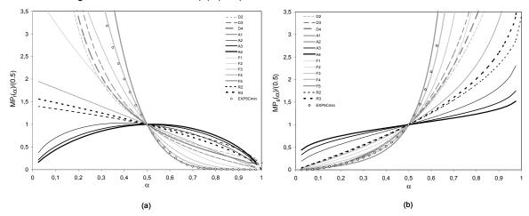
Figure 4. Master Plots based on the differential- $MP_f$  (a) and integral- $MP_g$  (b) form of the general law compared to the experimental data obtained by the thermal process applied (circles). Kinetic models: Dn: diffusion controlled, dashed lines, An: nucleation and growth, solid black lines, Fn: n-order reactor, solid grey lines, Rn: reaction controlled, pointed lines)
