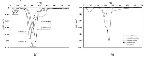
Figure 2. Comparison of DTG curves for rice straw at different atmospheres and heating rates (a) - Deconvolution curves for rice straw at 20°C/min using Ar as carrier gas (b)
