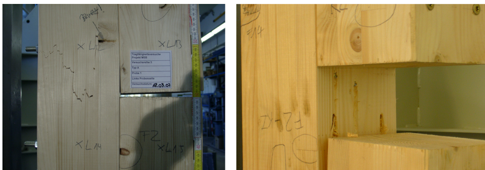
Figure 9: Exemplary states of fracture of one-sided fish-plate joints connected with dowel (left) and with continuously-threaded screws (right)
