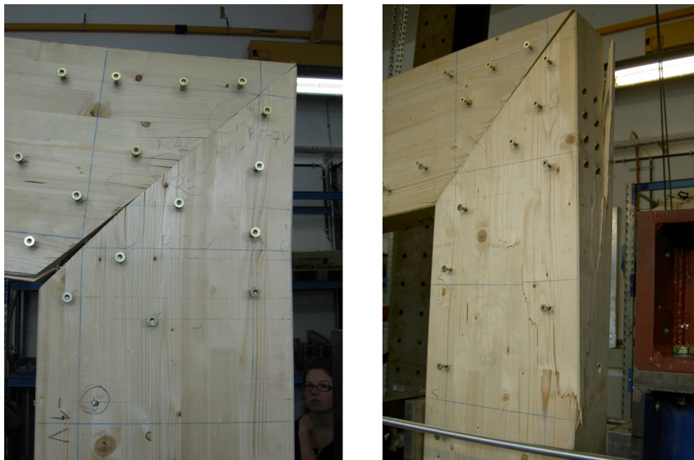
Figure 12: Failure of rigid frame corners connected with screws: left under positive moment, right under negative moment
