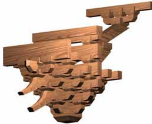
Figure 9: FEM solid model for 3 stepped bracket complex
