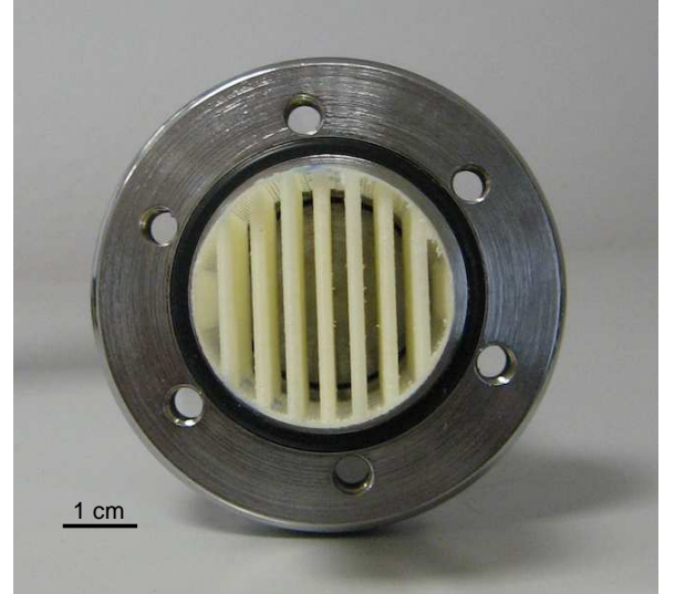
FIG. 4. (Color online) Photograph of a confined sonic crystal sample inside an acoustic impedance tube. The plastic sheath surrounding the sonic crystal allows its insertion in the tube.
