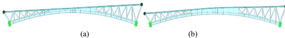
Fig. 6 Hybrid structure of arch and truss
