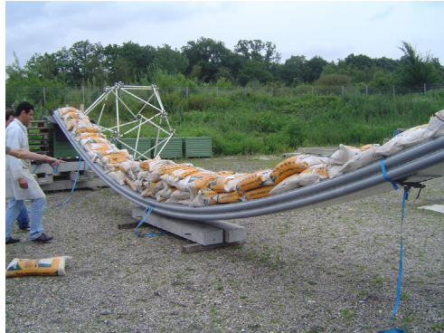
Figure 11. Loaded elements while the waiting for the resin to set up
