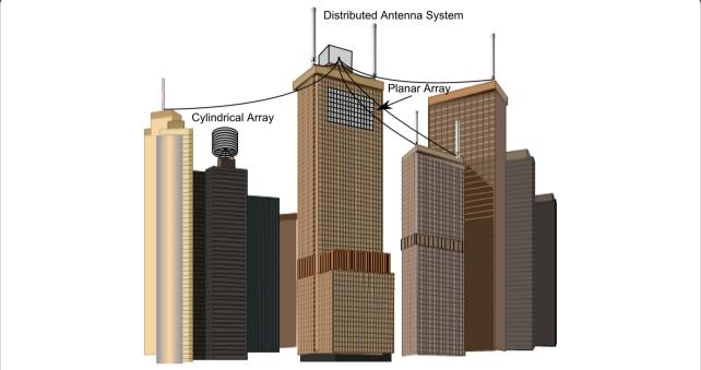
Figure 7 Different alternatives for the deployment of massive MIMO, including distributed antennas, planar arrays and cylindrical arrays.
