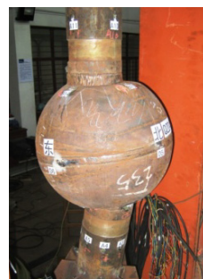
Fig. 4-4 Torsional failure modes
