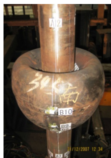
Fig. 4-3 Central failure modes
