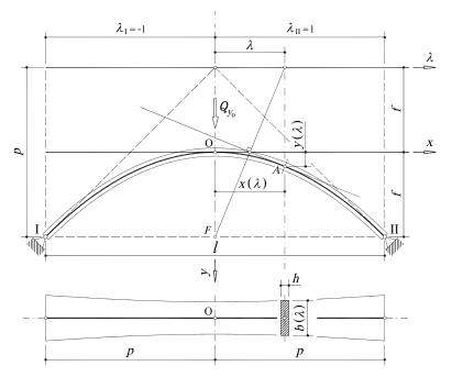
Figure 2: Hinged parabolic arch with hyperbolic variable cross-section.
