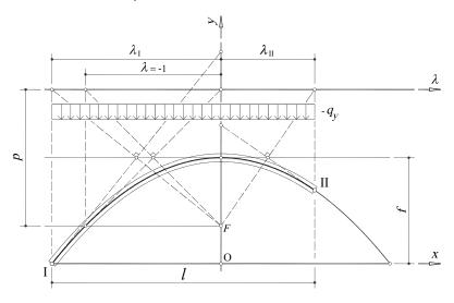
Figure 4: Parabolic arch with constant cross-section vertically loaded. The differential system Eq. (4) in this example, will be:
