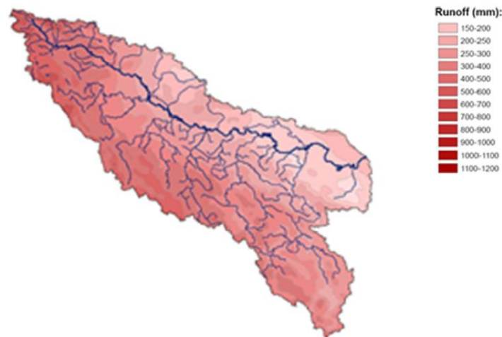
Figure 2.14: Mean annual runoff in the Sava River Basin (The Danube and its Basin – Hydrological Monograph, 2006).
