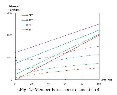
The fig.5 is a graph shows the element no.4's force in cable out of lower cables that get pretension. It is clear that the graph shows the nonlinear behavior in terms of member force, and as the load increases, the difference between them become more clear. With an supposition that the structure has no loading, there is no member force, when there is no pretension force is applied to the structure.
