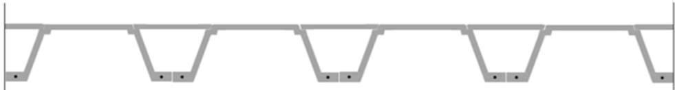
Figure 10: Transversal section of the flat roof, including the 20 mm thick plates disposed for create continuity between structural elements
