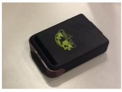
Fig. 20. GPS UMTS tracker with 48 hours of autonomy
