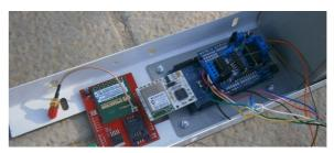
Fig. 19. Basic electronic modules placed on watertight internal structure
