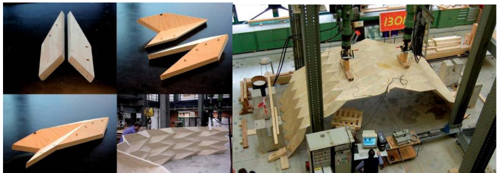
Figure 2: Digital chain and automotive production of folded plate structures
