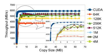
Fig. 4. Bandwidth test for copies from host to device with pinned host memory, using both native CUDA and the rCUDA framework over InfiniBand FDR, with different pipeline block sizes.
