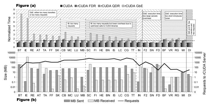
Fig. 8. (a) CUDA SDK samples normalized execution time using CUDA and rCUDA over different networks. (b) rCUDA profiling measurements for CUDA SDK samples. Primary Y-axis shows MB sent/received by samples to/from server when using the rCUDA framework. Secondary Y-axis presents requests sent to the rCUDA server. Both Y-axes in logarithmic scale.
