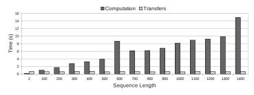
Fig. 14. NVIDIA profiling result for GPU-BLAST executing queries of different sequence lengths. In particular, time employed by computations (i.e., CUDA kernels) and memory transfers (i.e., CUDA memcopy).
