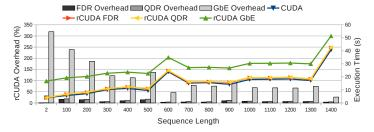
Fig. 12. GPU-BLAST execution time for queries of different sequence lengths, using CUDA and rCUDA over different networks. Primary Y-axis shows rCUDA's overhead, while secondary Y-axis represents execution time.
