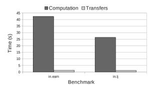
Fig. 16. NVIDIA profiling result for LAMMPS executing benchmarks in.eam and in.lj, scaled by a factor of 5 in all three dimensions. Time employed by computations (i.e., CUDA kernels) and by memory transfers (i.e., CUDA memcopy) is shown.
