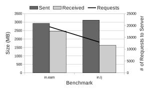
Fig. 15. rCUDA profiling measurements for LAMMPS executing benchmarks in.eam and in.lj, scaled by a factor of 5 in all three dimensions. Primary Y-axis shows MB sent/received by LAMMPS to/from server when using the rCUDA framework. Secondary Y-axis presents requests sent to the rCUDA server.
