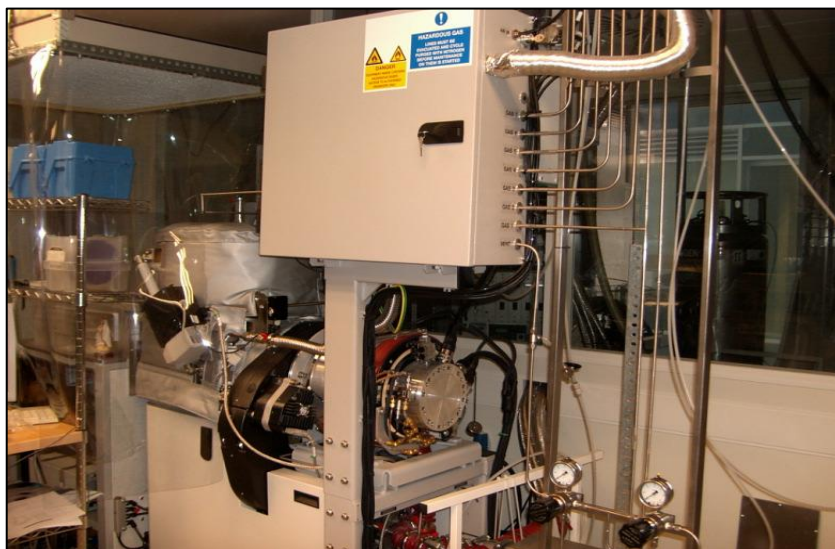
Figura 3.9 – Reactive Ion Etching with Inductived Coupling Plasma Source. Fuente: Elaboración propia.
