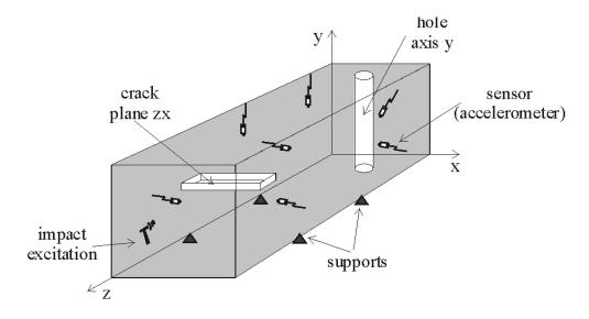
Figure 3. Setup experiment for a piece with a hole and a crack.
