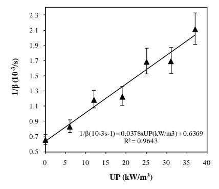
FIG. 6. Influence of ultrasonic power density on kinetic parameter  $1/\beta$  of eggplant cylinders at 1 m/s. Average values  $\pm$  LSD intervals (p<0.05).
