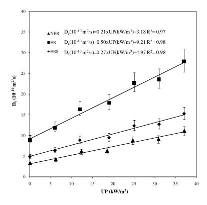
FIG 4. Influence of the ultrasonic power density (UP) on the mass transfer coefficient. Average values  $\pm$  LSD intervals (p<0.05).
