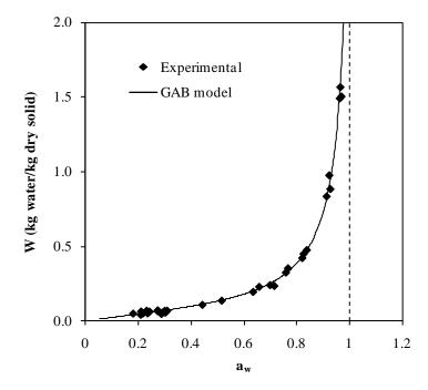
FIG.1. Experimental sorption isotherm and estimated curve with GAB model at 40 °C.
