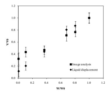
FIG. 2. Experimental shrinkage data for eggplant drying. V: Volume (m³), W: Average moisture content (kg water/kg dry solid), subscript 0: Initial. Standard deviation values.
