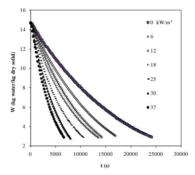
FIG 3. Drying kinetics of eggplant cylinders at 40°C and 1 m/s applying different ultrasonic power levels (kW/m³).
