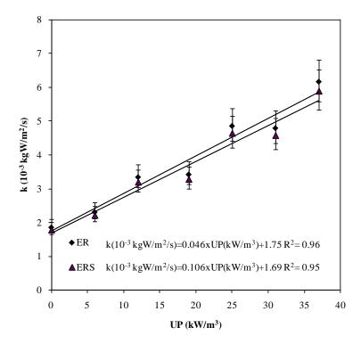
FIG 5. Influence of the ultrasonic power density (UP) on the mass transfer coefficient. Average values  $\pm$  LSD intervals (p<0.05).
