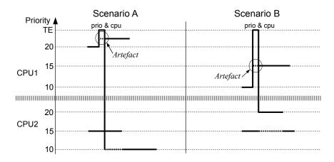
Fig. 3. An implementation based on a timing event prevents the scheduling errors shown in Figure 1. TE represents the priority at which the timing event handler is executed. In practice, under the Ceiling Locking policy, this priority is Interrupt\_Priority'Last.
