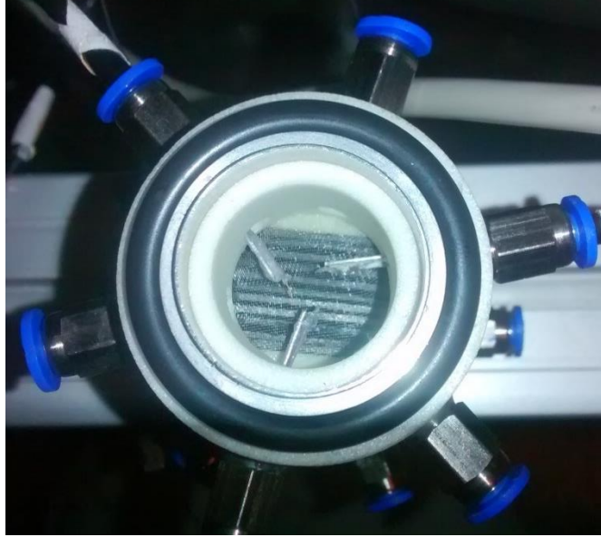
Fig. 3.2. Top view of the parallel-plate Gd regenerator inside the housing and thermocouples at the outlet section.
