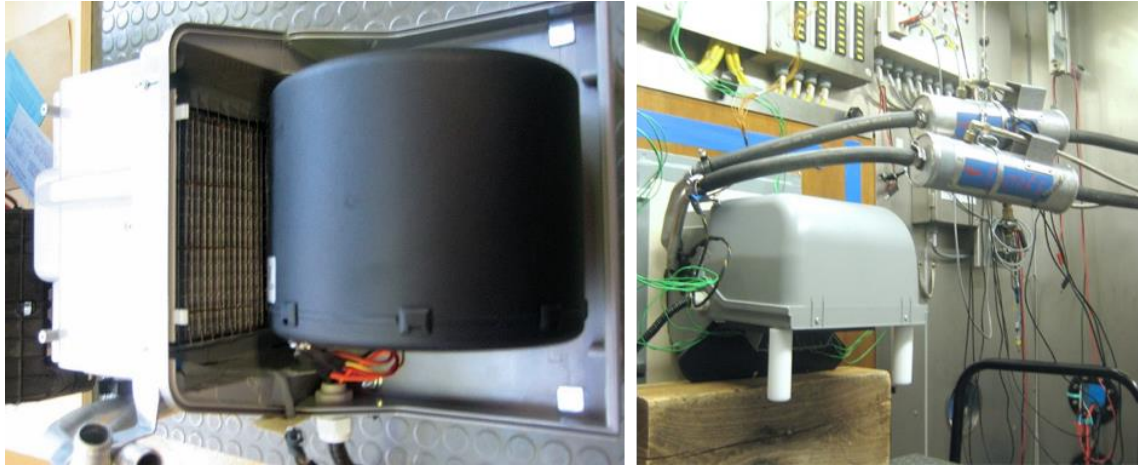
Fig. 5.14. Experimental setup: HEX inside HVAC unit (left) and HVAC unit in the test bench (right) [157].
