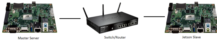
Figure 3.2: System composed of two Nvidia Jetsons TK1.
