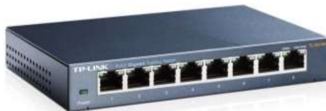
Figura 4: TP_LINK TL-SG108 Switch.
