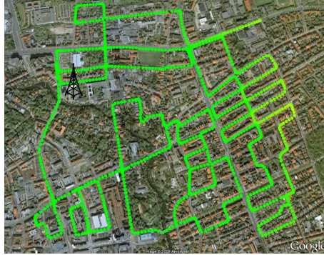
Figure 4.5: Map of Braunschweig with the position of the DVB-H transmitter and the considered streets in the simulations. Shown area is 2 km x 2 km.
