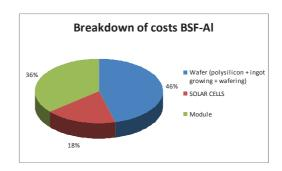
Fig. 7. Breakdown of module cost for BSF-Al technology.
