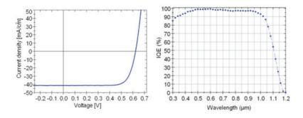
Fig. 2. Iluminated IV-curve and spectral response (IQE) of the best IBC solar cell with an efficiency of 19.6%.
