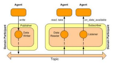
Fig. 1. Overview DCPS components from the DDS model.
