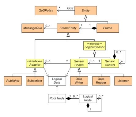
Fig. 2. UML class diagram of the middleware with the ontology support.
