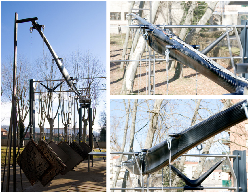
Figure 4: Full-size prototype beam during testing.
