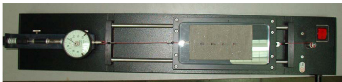
Figure 7. Device used to determine the static friction coefficient of the elastomer interlayer
