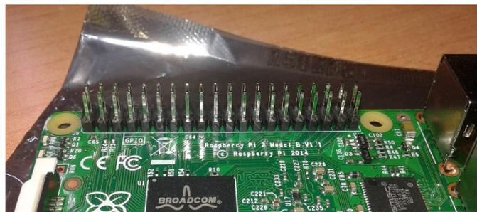
Fig. 75: Pins GPIO (1)
