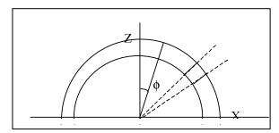
Figure 10: Section parallel to the XZ-face. For the meridians the angles φ of the normal lines with the Z-axis do not vary.
