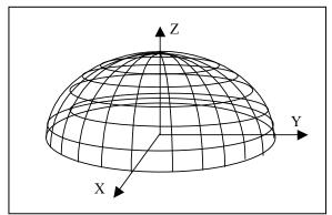
Figure 1: The globe-grid. The meridians are jointed at the top and the parallels are ellipses constructed in faces parallel the ground face.
