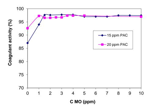
Figure 3. Results of Jar test using PAC and Moringa in type 1 water
