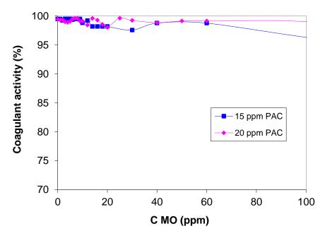
Figure 7. Jar test results for water type 2, using PAC as coagulant and a MO as coadyuvant
