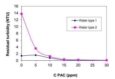
Figure 5. Results for Jar test with water type 1 and water type 2
