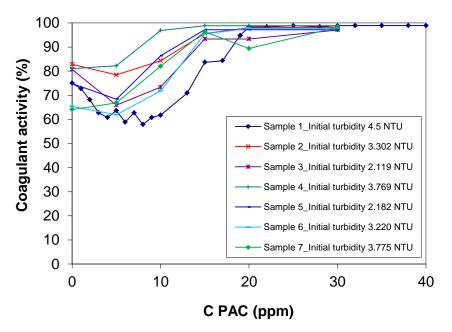
Figure 2. Results of Jar test using PAC as coagulant with type 1 water
