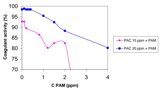
Figure 4. Results of Jar test using PAC and PAM in type 1water
