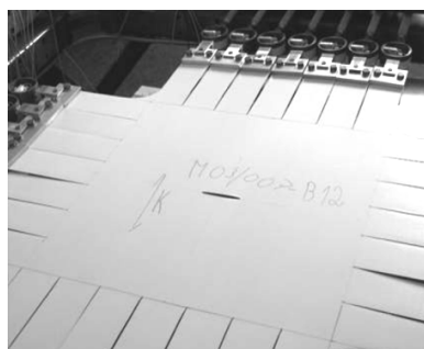
Figure 10a. Biaxial wide panel tear test Figure 10b. Test reduction due to slit length
