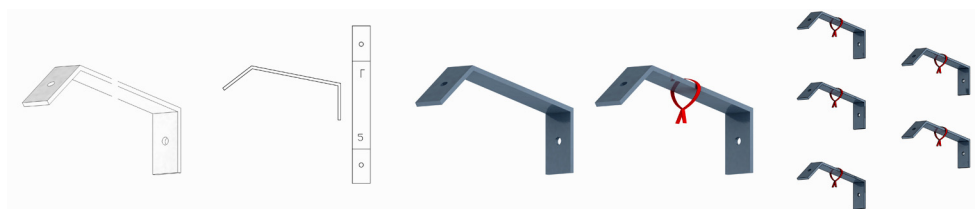
Figure 15: Typical design and construction process for a suspension bracket
