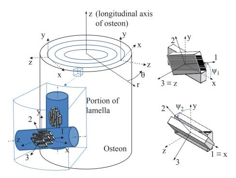
Figure 6: Coordinate system scheme. The local coordinate system (1, 2, 3) is aligned with each mineralized fibril. The cylindrical coordinate system  $(r, \theta, z)$  is used as a global coordinate system and a local auxiliary coordinate system (x, y, z) is defined at any point, being (x, y, z) coincident with  $(\theta, z, r)$  respectively. Definition of angles  $\psi_1$  and  $\psi_2$  that determine the crystal orientation.
