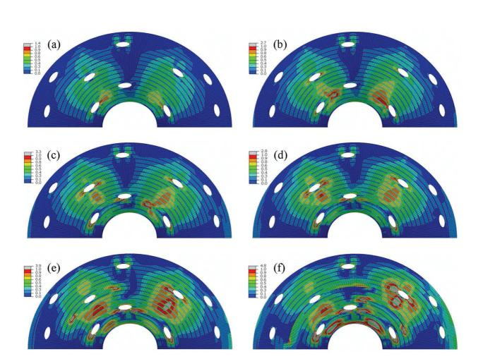
Figure 13: Node release technique. Evolution of the Brewer and Lagacé criterion for six instants of the microcracks initiation and propagation sequence. The instants correspond to the following applied pressures: (a)  $p \approx 14.0$  MPa, (b)  $p \approx 16.6$  MPa, (c)  $p \approx 18.0$  MPa, (d)  $p \approx 18.1$  MPa, (e)  $p \approx 19.1$  MPa, (f)  $p \approx 20.1$  MPa.
