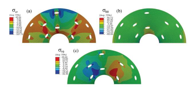
Figure 11: Stress fields (a)  $\sigma_{rr}$ , (b)  $\sigma_{\theta\theta}$  and (c)  $\sigma_{r\theta}$  for the failure initiation load of  $p \approx 14$  MPa, shown in Fig. 10.
