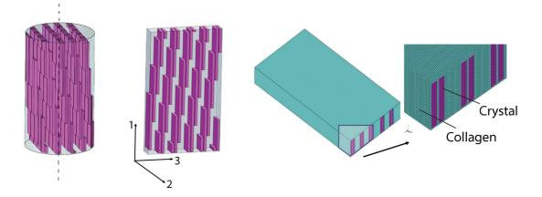
Figure 5: Representative volume element of a typical fibril structure modelled using finite elements by imposing periodical boundary conditions. The local coordinate system (1, 2, 3) is associated with the fibril orientation.
