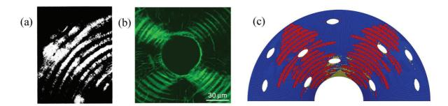
Figure 19: (a) and (b) Experimental images showing the damage in an osteon resulting from a radial compressive load, reported in Ascenzi et al. (1973) and Ebacher et al. (2012), both reprinted with permission of Elsevier. (c) Fields of progressive damaged elements for an advanced load state. In red, damaged elements according to the interlaminar failure criterion of Brewer and Lagacé (7); in yellow, damaged elements according to the intralaminar criterion (6).
