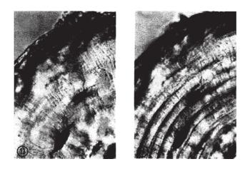
Figure 4: Behavior under compressive load of an osteon type I: left, before the loading; right, after the loading, showing the generation of microcracks. Reprinted from Ascenzi et al. (1973) with permission of Elsevier.
