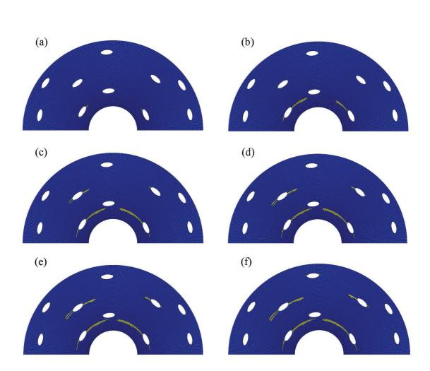
Figure 15: Progressive damage approach. Evolution of damaged elements (shown in yellow) by application of the interlaminar failure criterion of Brewer and Lagacé (7) for six instants of the damage propagation sequence. The instants correspond to the following applied pressures: (a)  $p \approx 14.0$  MPa, (b)  $p \approx 16.6$  MPa, (c)  $p \approx 18.0$  MPa, (d)  $p \approx 18.1$  MPa, (e)  $p \approx 19.1$  MPa, (f)  $p \approx 20.1$  MPa.
