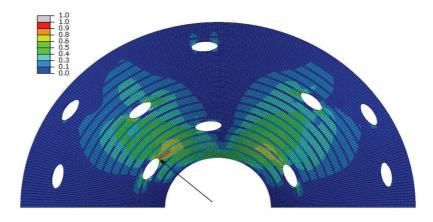
Figure 10: Initiation criterion. Application of the failure criterion of Brewer and Lagacé to determine the initiation of failure, reached at a load of  $p \approx 14$  MPa.
