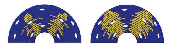
Figure 16: Progressive damage approach. Damaged elements (shown in yellow) by application of the interlaminar failure criterion of Brewer and Lagacé (7) for two advanced loading states (left,  $p \approx 29.3$  MPa; right,  $p \approx 31.5$  MPa.
