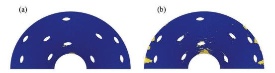
Figure 17: Progressive damage approach. Evolution of damaged elements (shown in yellow) by application of the intralaminar failure criterion (6) for two instants of the damage propagation sequence.
