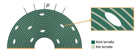
Figure 9: Finite element model, showing the applied load, the displacement constraints, the lamellae and the lacunae considered. The mesh is structured, enabling the arrangement into thin and thick lamellae of constant thickness and the cylindrical orientation of the material axis for each lamella. The detailed view shows the modification of the structured mesh to allow for the presence of lacunae.
