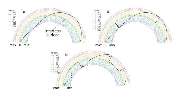
Figure 12: Node release technique. Evolution of shear stress along one of the contact surfaces (CSHEAR in Abaqus). For the sake of clarity, the surface does not intersect any lacunae. (a) Stress state before microcrack initiation; (b) microcrack initiation; (c) microcrack propagation.
