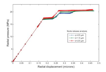
Figure 14: Node release technique. Sensitivity analysis to the characteristic length d used in the application of the procedure.
