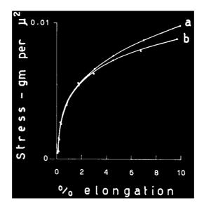
Figure 8: Stress-strain curves for tensile tests in the z-axis of single osteons. Curve (a) corresponds to a wet and fully calcified type I osteon, taken from a man of 30. Curve (b) Same from a man of 80. Note:  $1 \text{ gr}/\mu\text{m}^2 \approx 10^4 \text{ MPa}$ . Reprinted from Ascenzi and Bonucci (1967) with permission of John Wiley and Sons.
