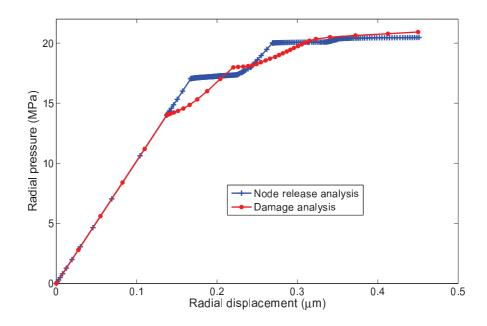
Figure 18: Comparative evolution of the applied pressure vs. the displacement of the load application point located on the vertical radius. Results for both techniques: node release technique and progressive damage approach.
