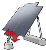
One axis polar tracker (inclined axis)
