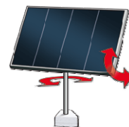
Two-axes tracker (Elevation / azimuthal)
