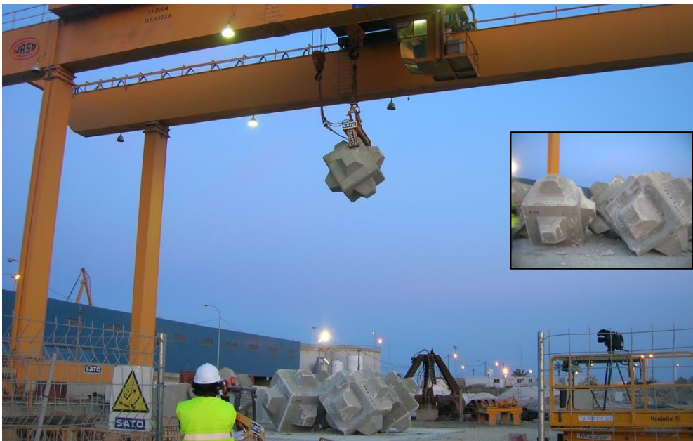
Figure 4.4 Sixteen-tonne Cubipod ® unit being dropped onto four Cubipods in an extreme free-fall test, h_c[m]=9.5 (EED).
