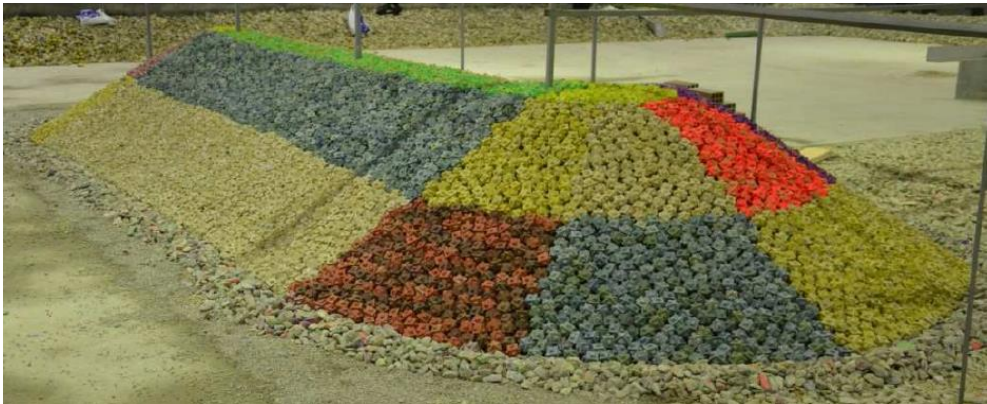
Figure 2.7a Double roundhead 3D model with single-layer Cubipod ® armor tested at UDC.
