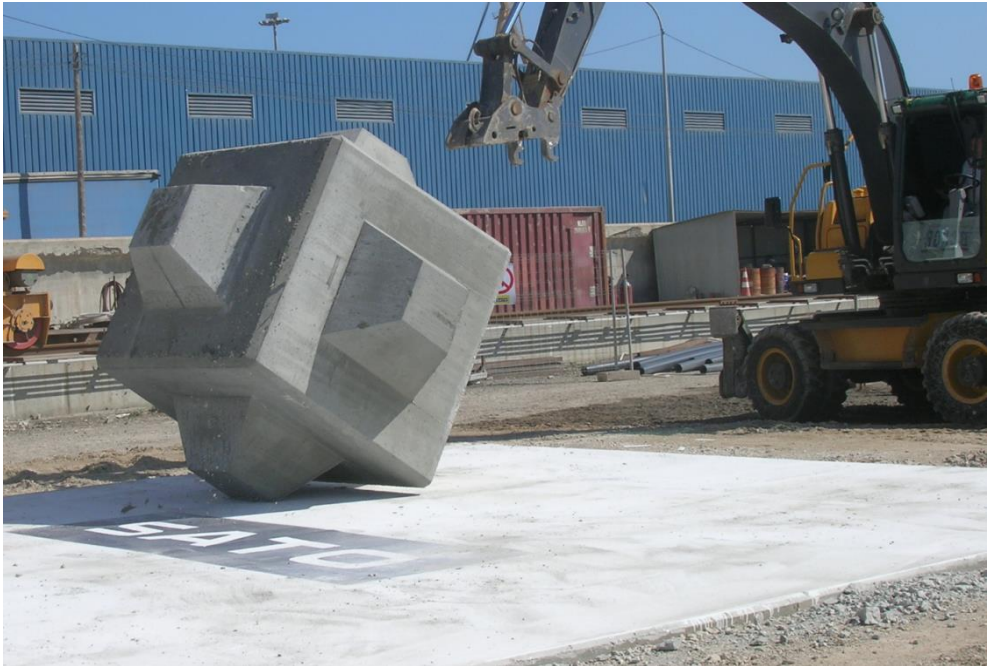
Figure 4.1 Steel-reinforced concrete overturning platform (10.0x7.5x0.9 m).
