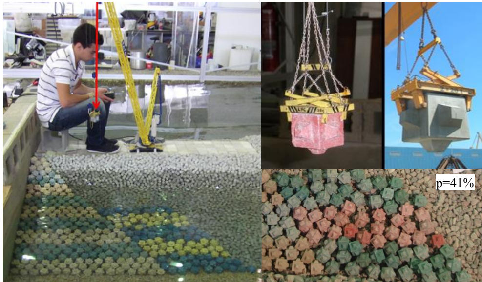
Figure 6.8 Realistic armor placement. Straight trunk.
