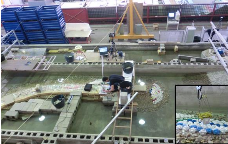
Figure 6.10 Small-scale realistic placement of Cubipods in trunk and roundhead.
