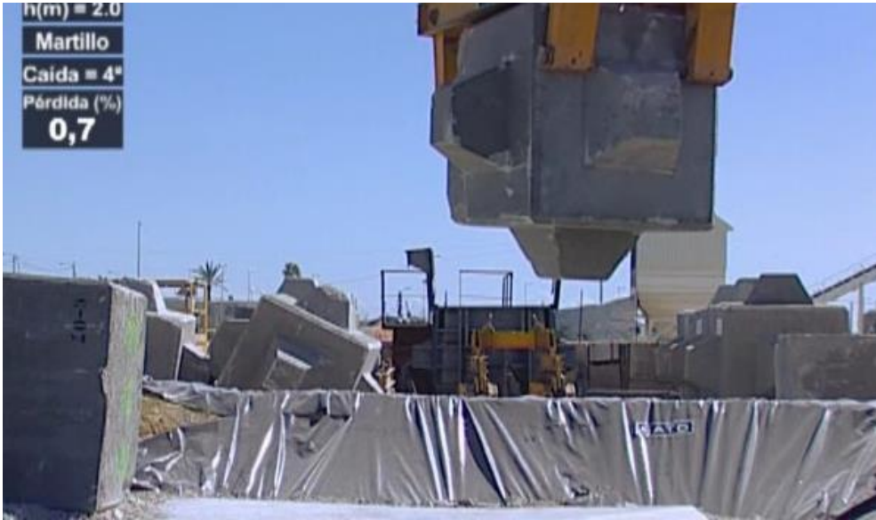
Figure 4.2 Cubipods dropped on the rigid free-fall platform (5.0x5.0x1.15 m).
