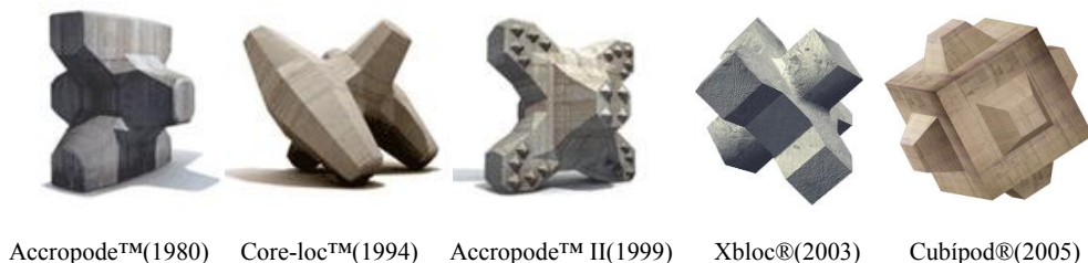
Figure 2.1 Units for single-layer armoring.
