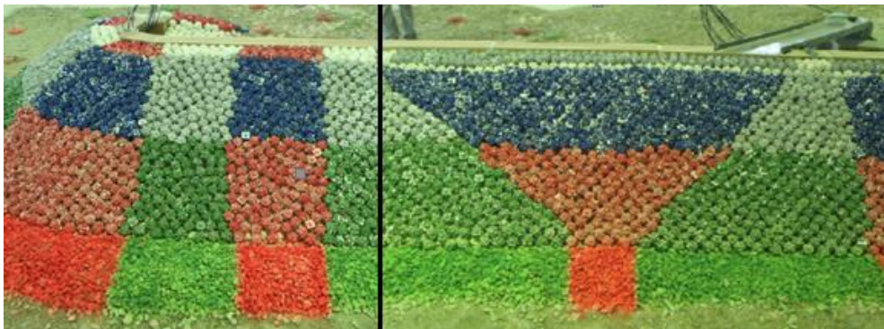
Figure 6.12 Transition single-to-double Cubipod ® armor.
