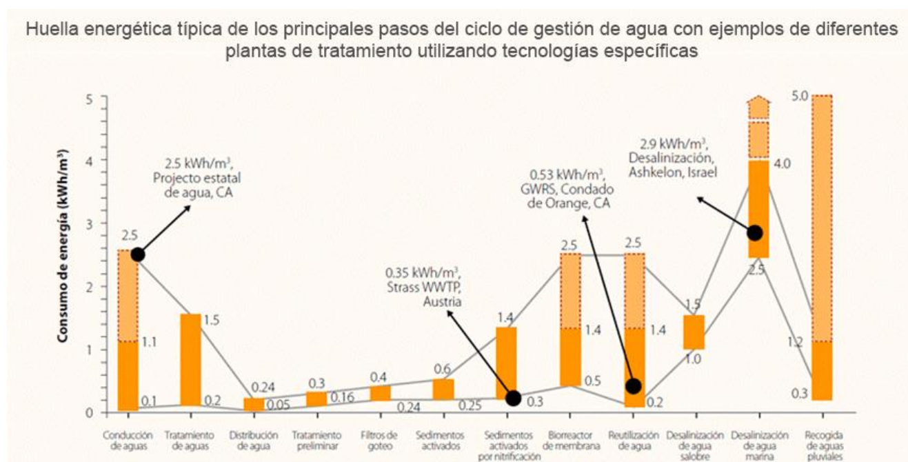
Figura 1-7: Consumos específicos de energía. Nota: GWRS, groundwater replenishment system; WWTP, wastewater treatment plant (Lazarova et al. 2012)
