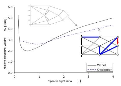
Figure 4: Comparison between the structural weight of Michell-Structures and the topology optimized adaptive truss structures under simultaneous force and deformation adaptation and a single load case
