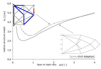
Figure 5: Comparison between the structural weight of Michell-Structures and the topology optimized adaptive truss structures under simultaneous force and deformation adaptation and single load case
