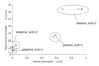
Figure 6: Comparison between the structural weight of Michell-Structures and the topology optimized adaptive truss structures under simultaneous force and deformation adaption and multiple load cases
